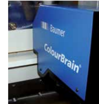
Inspection of laminated edges.
