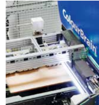
Double sided inspection of body elements.
