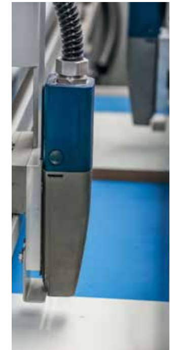
Marking a defect on protective foil.
