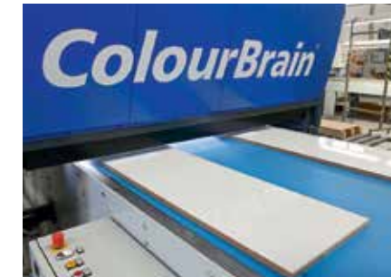
Installation in the lacquering line.
