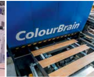
Automatic inspection of floor planks.
