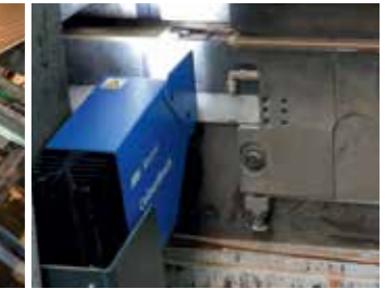
Automatic inspection of edge laquering.
