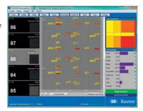
The user deploys an intuitive user interface that is easy to understand with clearly structured graphical menus. ColourBrain® gives precise documentation of position of defects on the web, crosswise and in machine direction.
